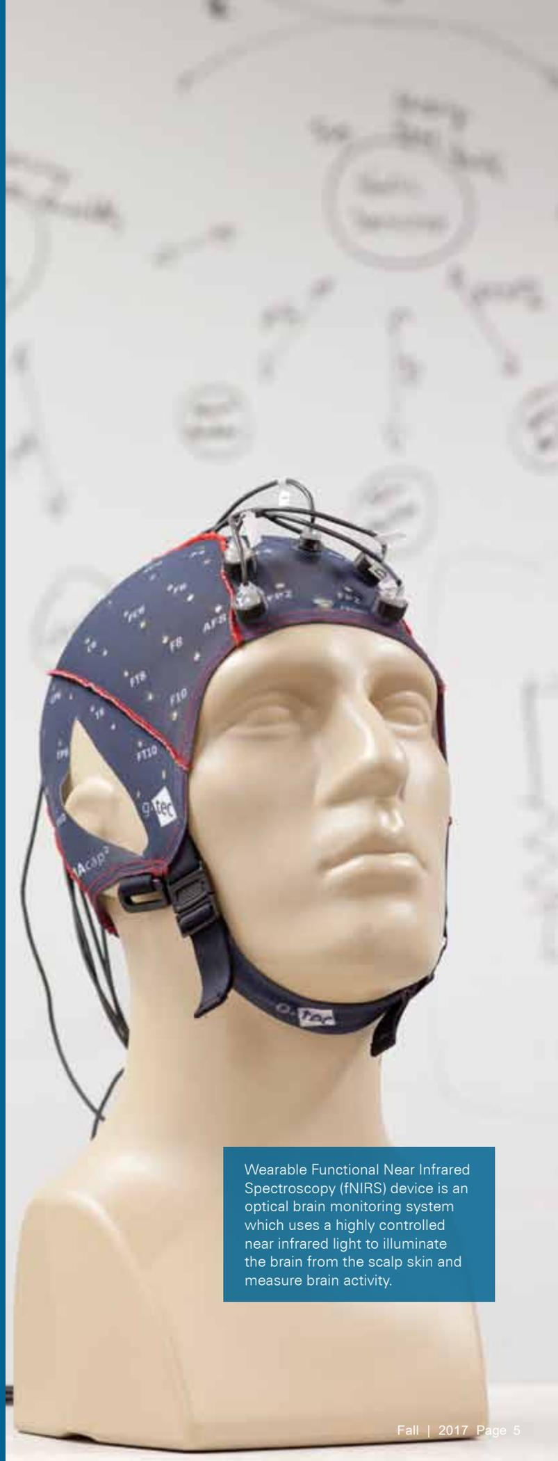
Wearable Functional Near Infrared Spectroscopy (fNIRS) device is an optical brain monitoring system which uses a highly controlled near infrared light to illuminate the brain from the scalp skin and measure brain activity.
