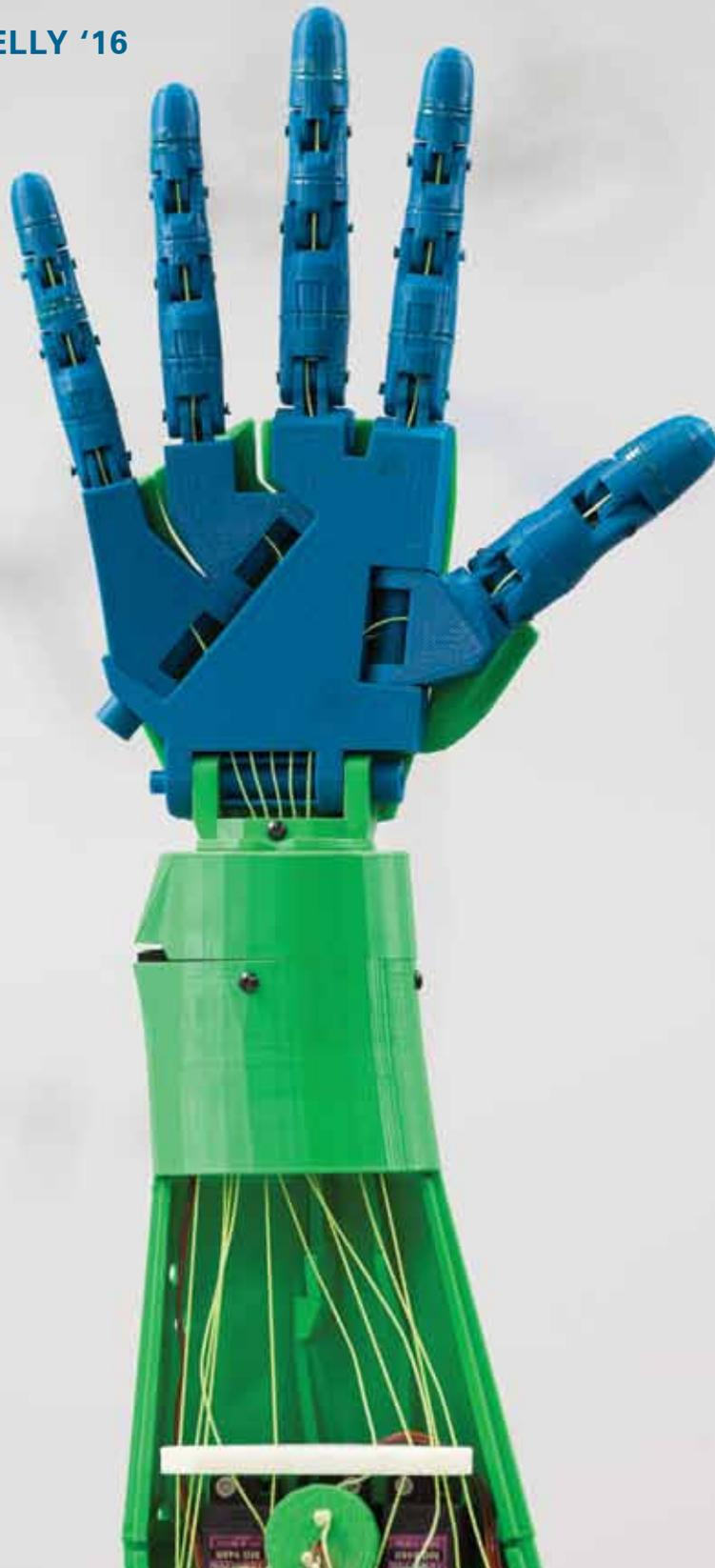
3D-Printed Robotized Hand, developed to help amputees.
