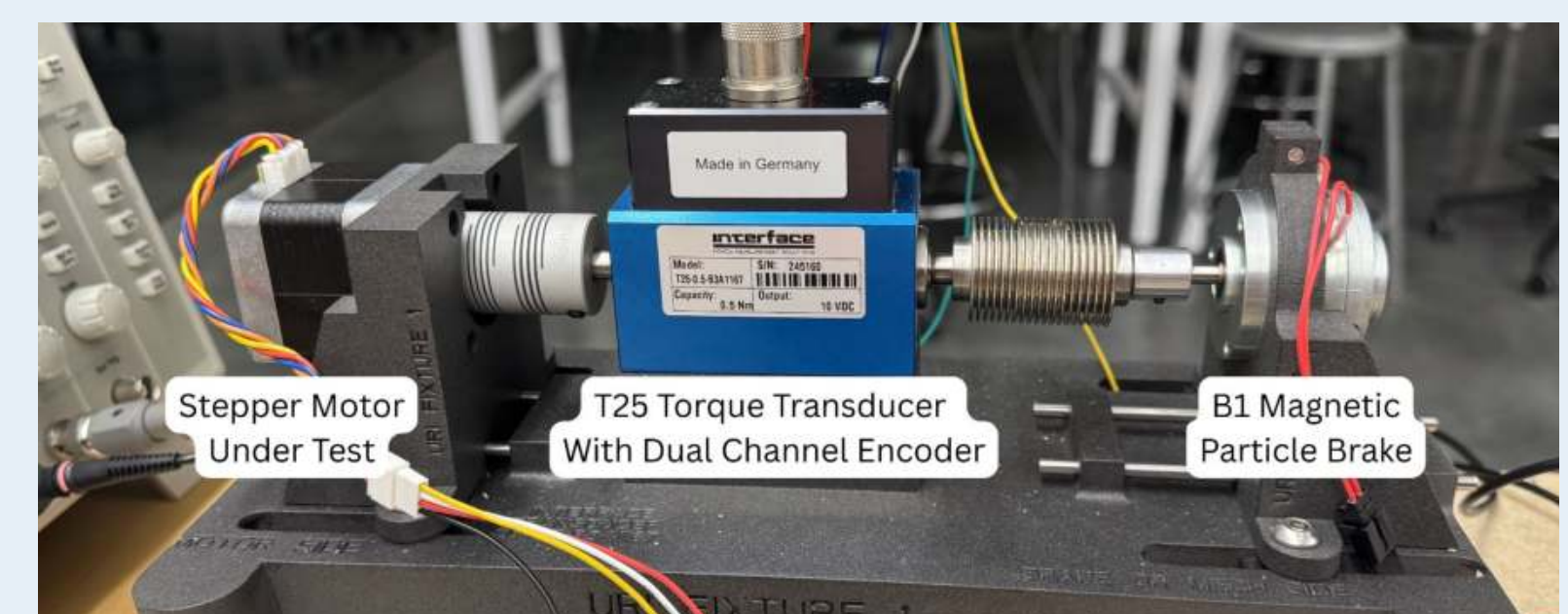
Fig. 1: Torque measurement test fixture including stepper motor, torque transducer, and magnetic particle brake
