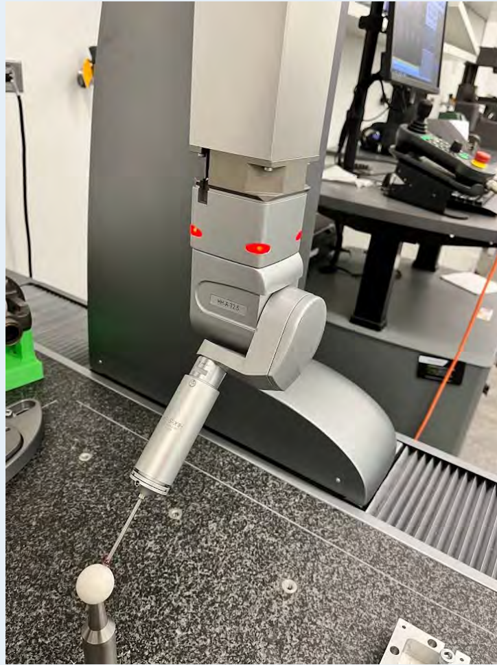
Figure 2: A-45B90: Rotation 90°, Tip Angle -45°
