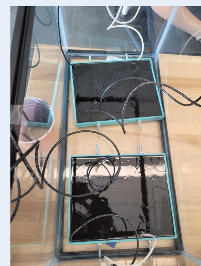
Fig. 3: Primary and secondary coils potted
