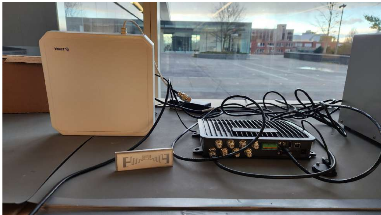
Figure 3: Photo of our lab setup. The white square is a fixed reader. The black box is an interface for us to read the data from the scanner. The small block is an antenna attached to a metal block to be read by the scanner.
