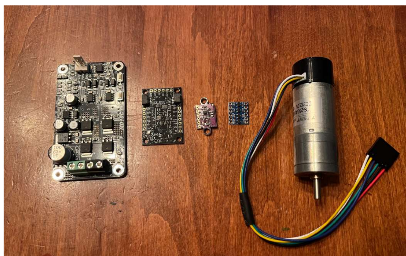
Figure 4 - Test Environment Components (Left to Right: Motor Driver, Gyroscope, Laser, Level Shifter, and Motor)
