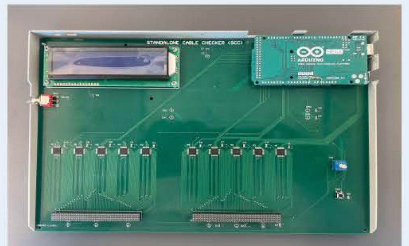
Figure 2: Assembled Main PCB (top)
