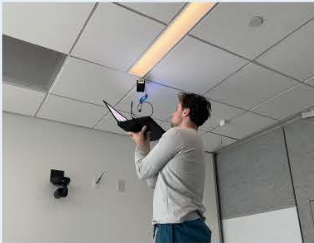
Fig. 4: Testing a PV cell at a specific angle with the PV Angler and Power Profiler Kit II
