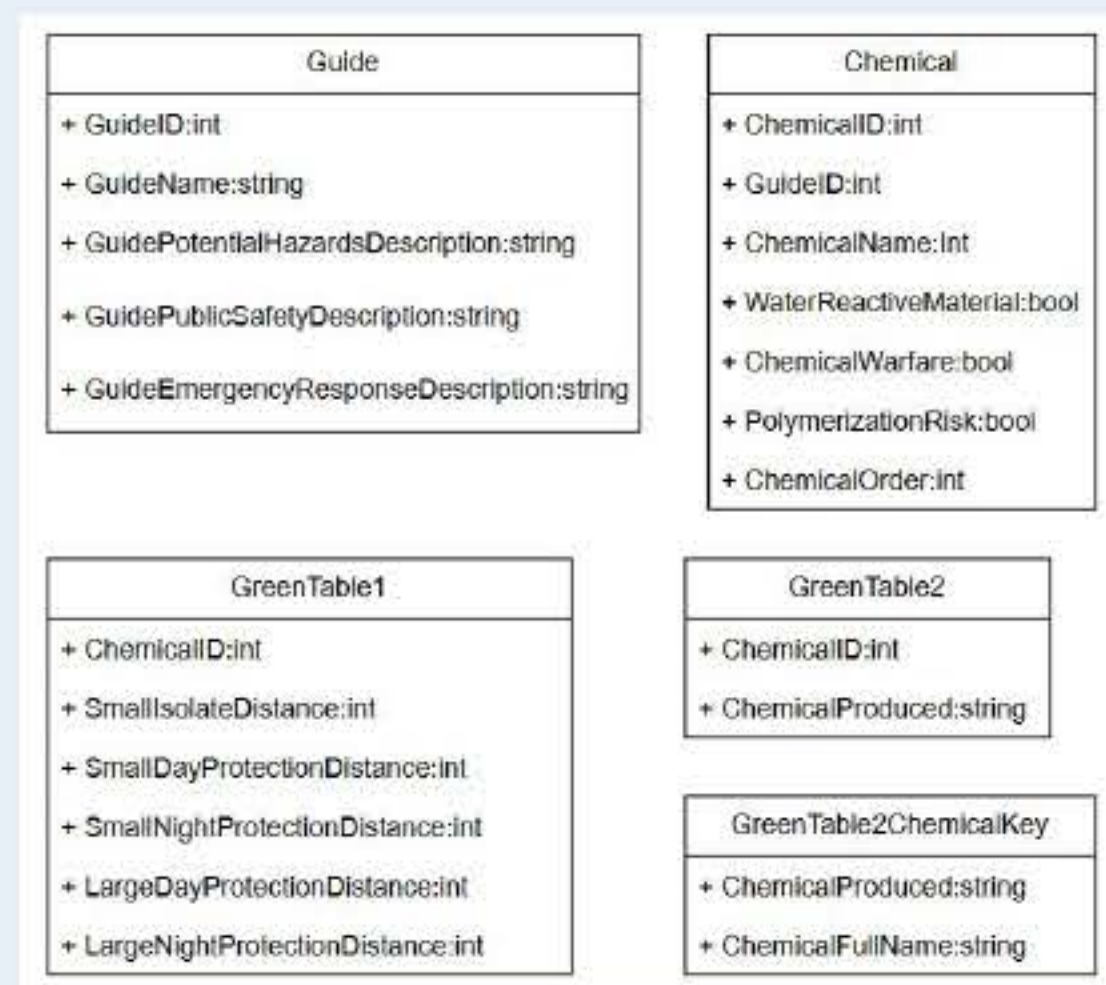
Fig. 2: Block diagrams of SQL database schema.
