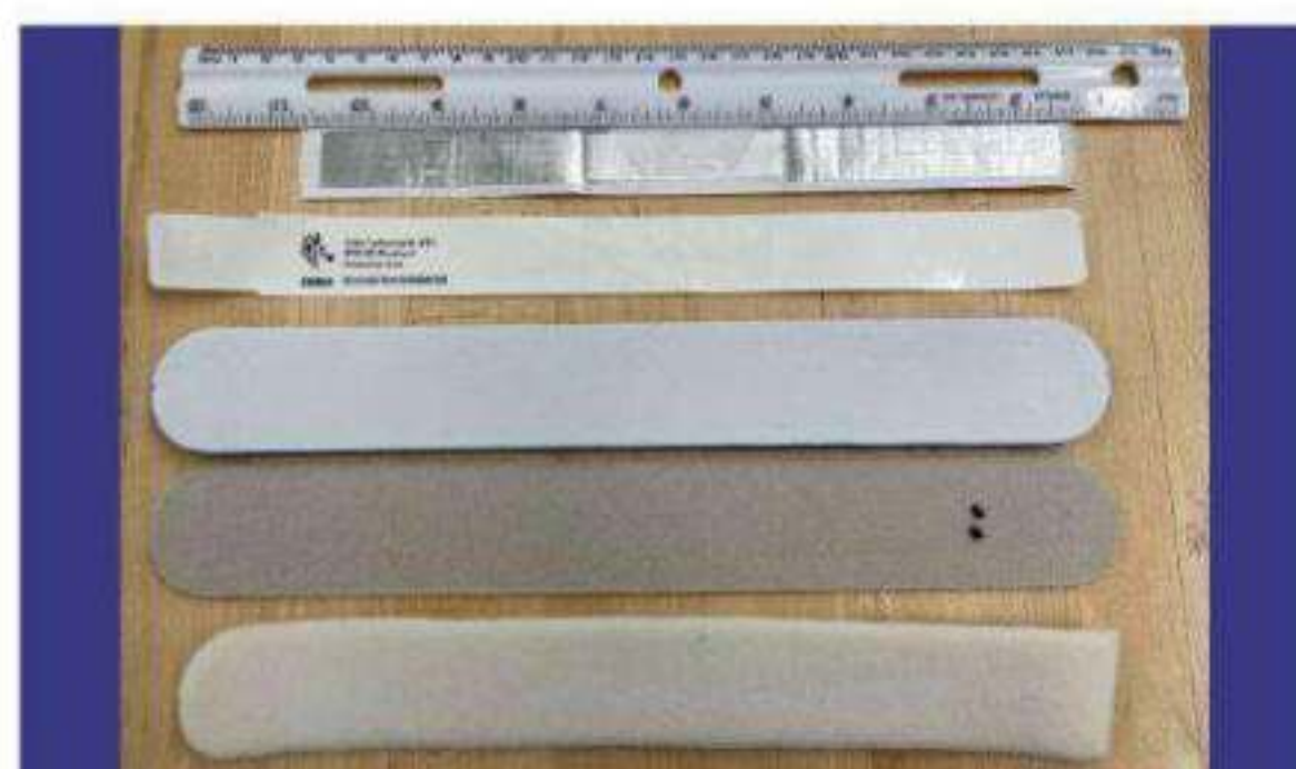
Figure 4: Top to Bottom: RFID Tag Antenna and Chip, Plastic Tag Cover, FabriFoam Nimbus, FabriFoam X-Treme, ComfyCuff
