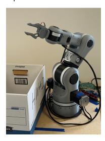
The arm itself consists of one servo motor (for the "hand") and several stepper motors (for the arm joints). These motors are all controlled by motor control modules, which are driven by an xcore.ai chip. The PCB also includes a second xcore.ai chip that is listening for voice commands to tell the arm where to go. This arm is a great demonstration of how flexible XMOS chips are, and that makes it a useful tool for sales and marketing.
