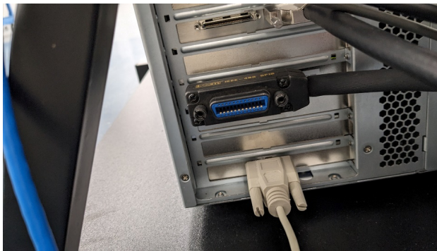
GPIB cable between computer and digital multimeter
