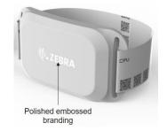
Once attached to a patient's wrist, the Beacon would continuously broadcast advertising packets with AoA CTE data every 1 to 2 seconds. The battery would be sized to last at least 14 days. There are no switches or LEDs on the wristband PCBA. The desire is to know with an accuracy of 99% which room the patient is in.
