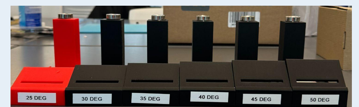
Fig. 3: PV Anglers, used for testing PV cell performance
