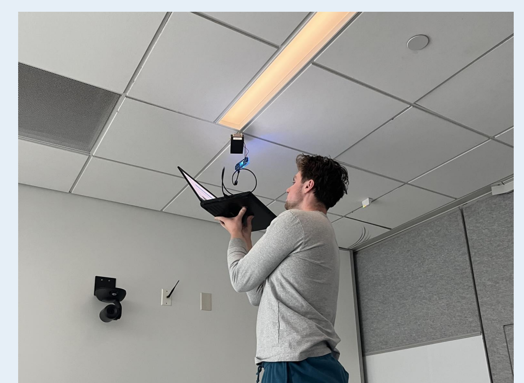
Fig. 4: Testing a PV cell at a specific angle with the PV Angler and Power Profiler Kit II
