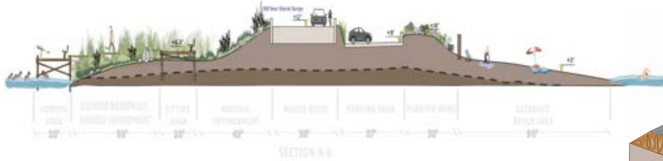
SECTION A-A OBSERVATION DOCK SECTION
