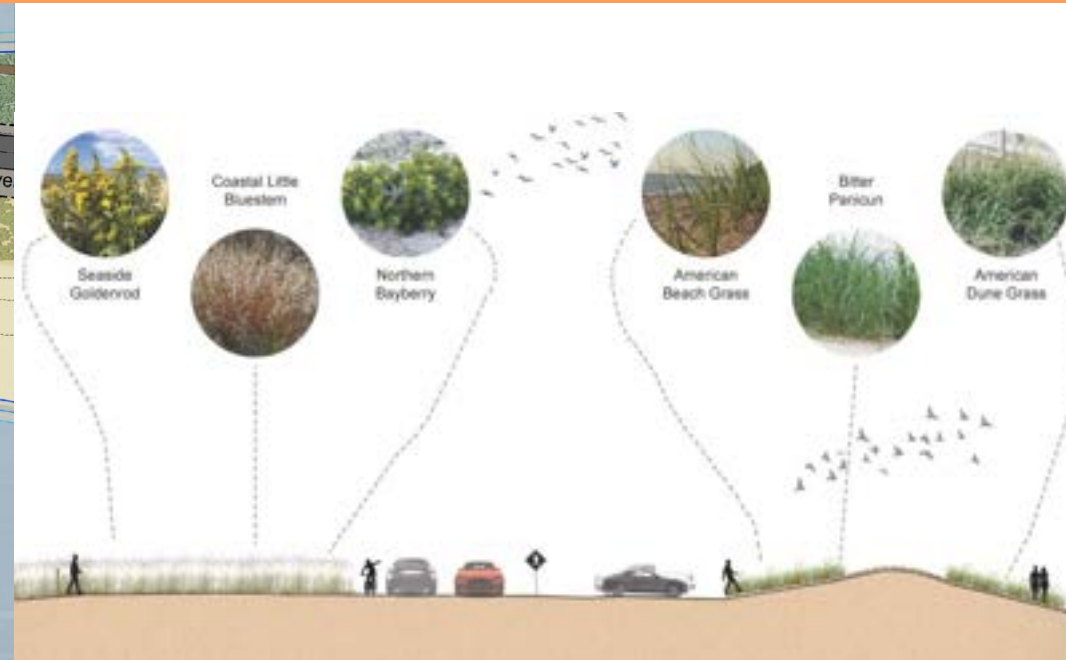
Dune Restoration and Plant Material Section
