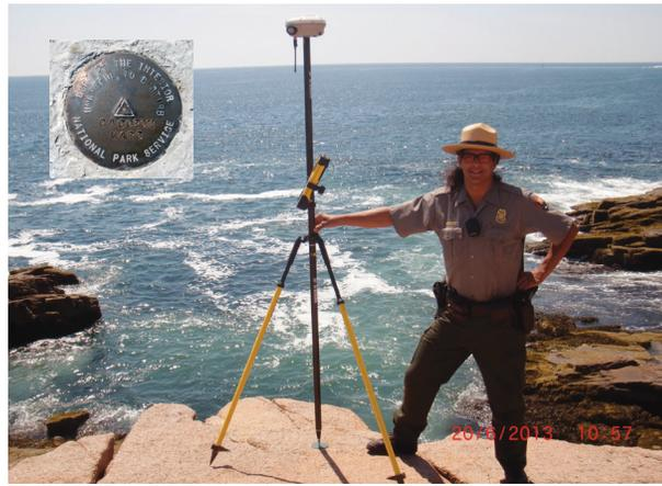
**Figure 2.** A park ranger uses a survey monument (beneath the center tripod leg), or benchmark, to position an RTK-GPS instrument. These monuments serve as stable reference points when collecting elevation data. Inset: Example of an embedded NPS survey monument, several inches in diameter. Photos courtesy of Michael Bradley, University of Rhode Island Environmental Data Center
