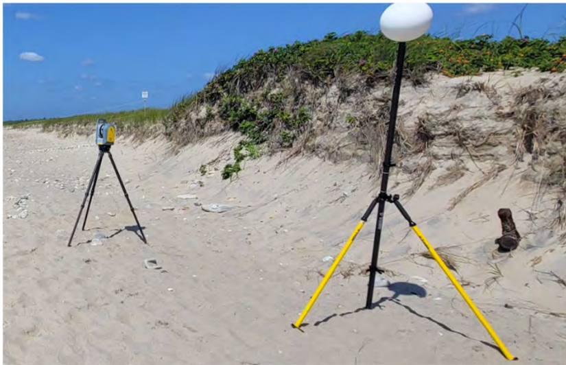
Terrestrial LiDAR setup
