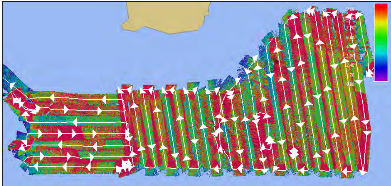
Figure 26. The Volcano South survey area, colored by sounding density. Large variations in speed resulted in variations in density along track. Main survey lines are typically broken automatically based on a specified time (30 minutes in this case, unless there was an issue or a planned turn), so longer lines generally indicate faster speed.
