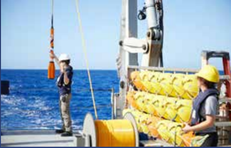
Marine Technician Karrel Kaspar leads the magnetometer deployment from Falkor's aft deck.
