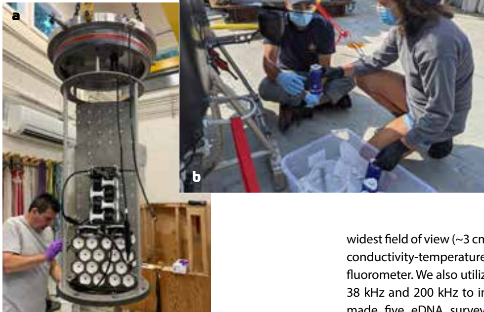
FIGURE 2. (a) WHOI mechanic Brian Durante conducts pressure testing of the eDNA sampler in Woods Hole. Photo credit: Lui Kawasumi. (b) WHOI research assistant Erin Frates and Oceanic Labs engineer Lui Kawasumi prepare the eDNA sampler. Photo credit: Dana Yoerger
