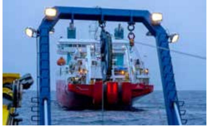
FIGURE 3. Cable Ship Cable Innovator is viewed here from the back deck of E/V Nautilus during a carefully choreographed dual-ship operation to lay 5 km of fiber-optic cable at Endeavour Ridge.
