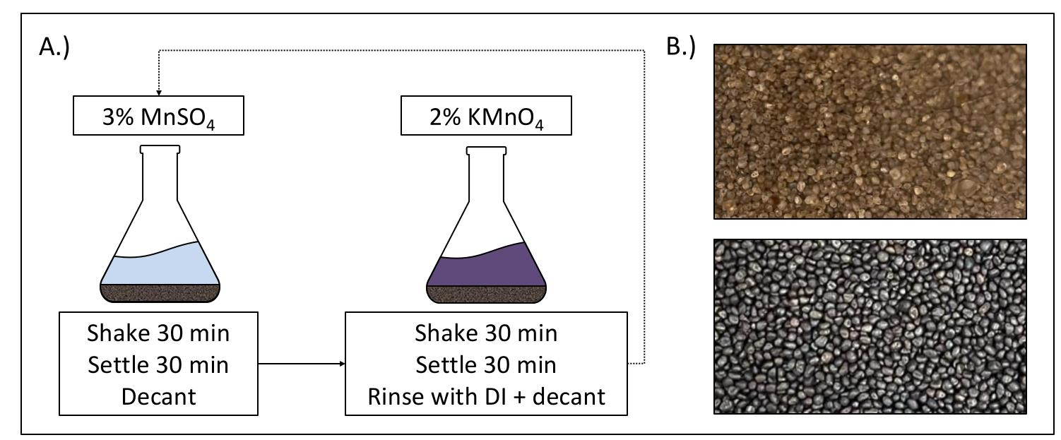
**Figure 1.** A.) Process diagram for media synthesis. Coating is applied to ~100 g of Ottawa sand. B.) Media prior to repetitive coating (top), and after (bottom).
