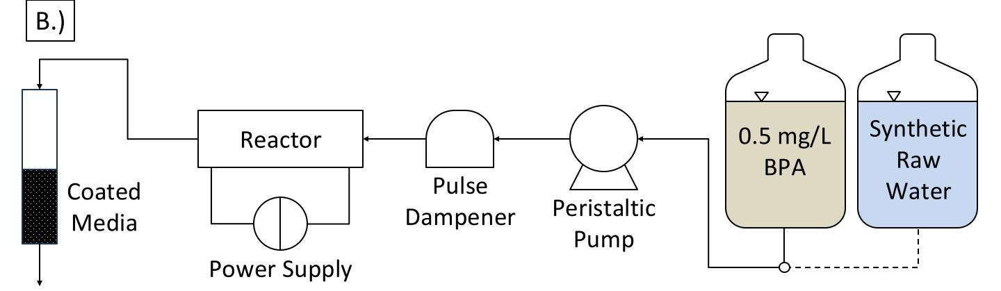
**Figure 2.** A.) Bench-scale setup for all detailed experiments (Figures 4-6). B.) Process diagram for setup shown in Figure 2A. For chemical regeneration (Figure 6A), reactor was disconnected.
