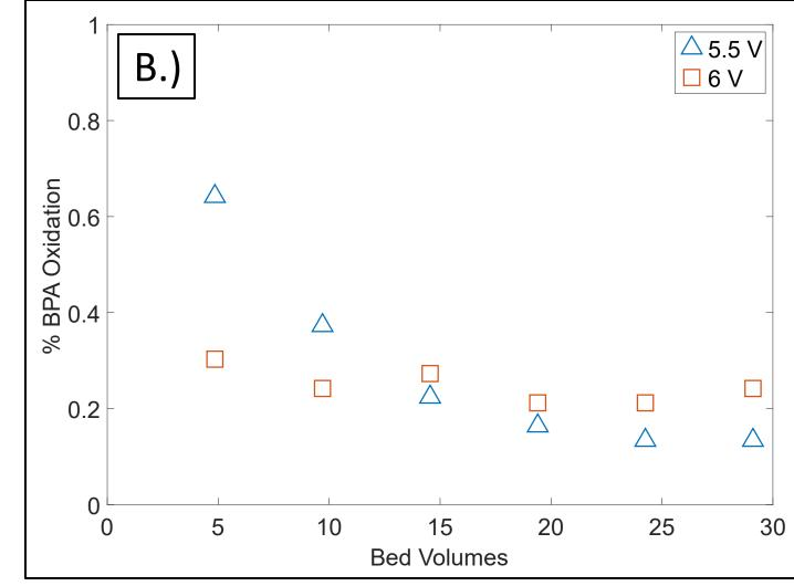
**Figure 6.** A.) Oxidation of BPA by  $MnO_x$ -coated media regenerated chemically. B.) regenerated electrochemically at 5.5 and 6.0 V (Figures 5A and B). Chemically regenerated media was run until the media was fully expended; electrochemically was not.
