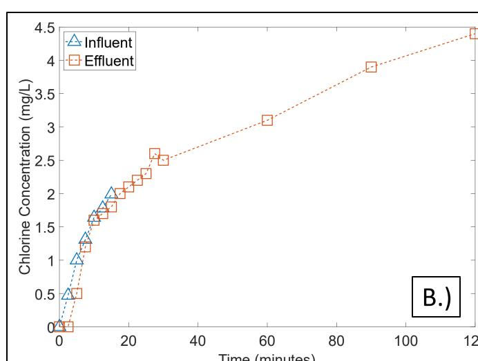
**Figure 5.** A.) Electrochemical regeneration of fully expended media via production of chlorine at 5.5 V for 40 minutes. B.) at 6.0 V for 2 hours.
