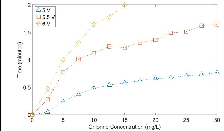
**Figure 4.** Chlorine influent produced by the reactor at 5, 5.5, and 6 V. Measurements for 6 V exceeded 2 mg/L after 15 minutes.
