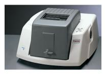
The Nicolet 380 FT-IR spectrometer is used to obtain an infrared spectrum of absorption or emission of a solid, liquid, or gas. Nicolet 380 is a reliable, easy-touse system that helps identify, quantify and verify samples.
