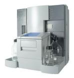
The Surface plasmon resonance instrument can be used to characterize molecular interactions between biomolecules ranging in size from ions to viruses.
