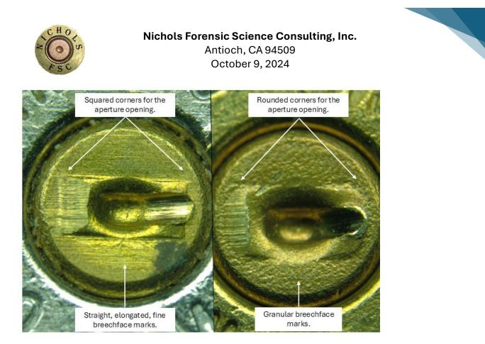
In addition, though they were not photographed, the firing pin impressions were also clearly different. Each of the two comparisons, the breechface marks and the firing pin impressions, required that the lighting be appropriately adjusted by putting the cartridge cases on a tilt. However, this is not an unusual technique and would be considered standard for a critical comparison of the marks.
