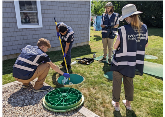
Collecting wastewater samples from a nitrogen reducing system
