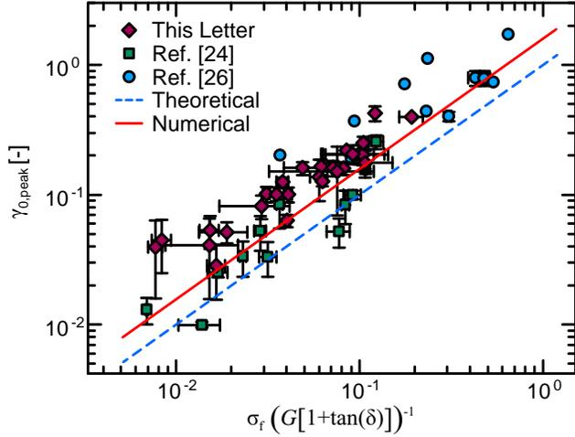
FIG. 4. Strain amplitude at the  $G''$  overshoot  $\gamma_{0,\text{peak}}$  as a function of the nondimensional parameter of flow stress  $\sigma_f$ , linear storage modulus  $G$ , and  $\tan(\delta)$ . Lines show numerical (red) and theoretical (blue) predictions.
