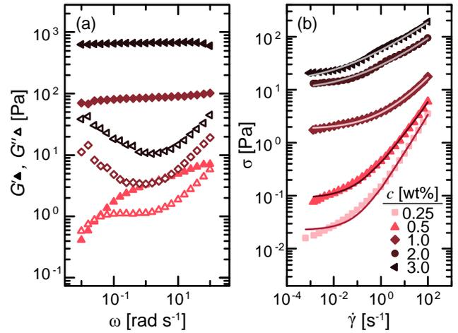
FIG. 1. (a) Storage modulus  $G'$  (closed symbols) and loss modulus  $G''$  (open symbols) as a function of oscillation frequency  $\omega$ . (b) Stress  $\sigma$  as a function of shear rate  $\dot{\gamma}$  for samples containing the specified concentration of POJO-250. Curves are fits to the Herschel-Bulkley model.
