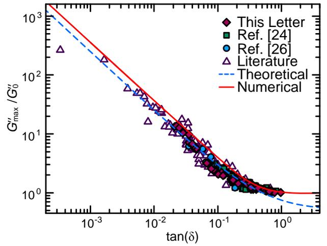
FIG. 3. Normalized magnitude of the  $G''$  overshoot ( $G''_{\max}/G''_0$ ) as a function of the LVR value of  $\tan(\delta)$ . Literature sources of yielding metrics are from Refs. [27–43] and are described in Supplemental Material [44]. Curves indicate numerical (red) and theoretical (blue) predictions based on the KDR model.
