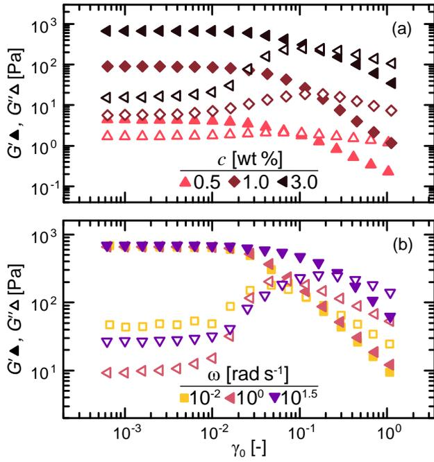
FIG. 2. Storage modulus  $G'$  (closed symbols) and loss modulus  $G''$  (open symbols) as a function of strain amplitude  $\gamma_0$  (a) for samples containing different polymer concentrations  $c$  at the same frequency  $\omega = 10 \text{ rad s}^{-1}$  and (b) for samples containing  $c = 3 \text{ wt\%}$  POJO-250 at different frequencies  $\omega$ .
