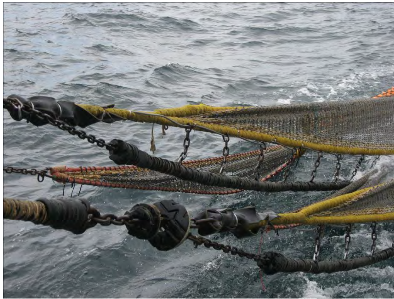
Figure 3. Photos of full scale MFN with (a) extensions on headrope and (b) 30.5 cm (12 in.) drop chains connected to footrope being deployed during field trials.
