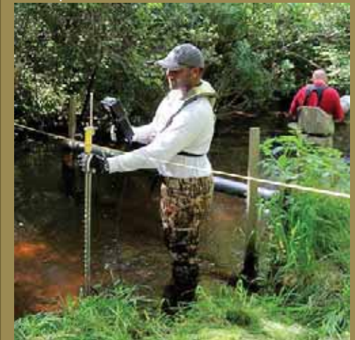
A USGS scientist measures stream flow. Photo courtesy of USGS.
