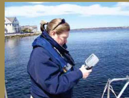
A scientist from NBC taking dissolved oxygen measurements using a YSI sonde. Photo courtesy of NBC.
