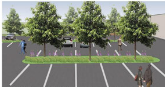
The Wharf Tavern parking lot with installed eco-swales containing vegetation, and permeable pavement
