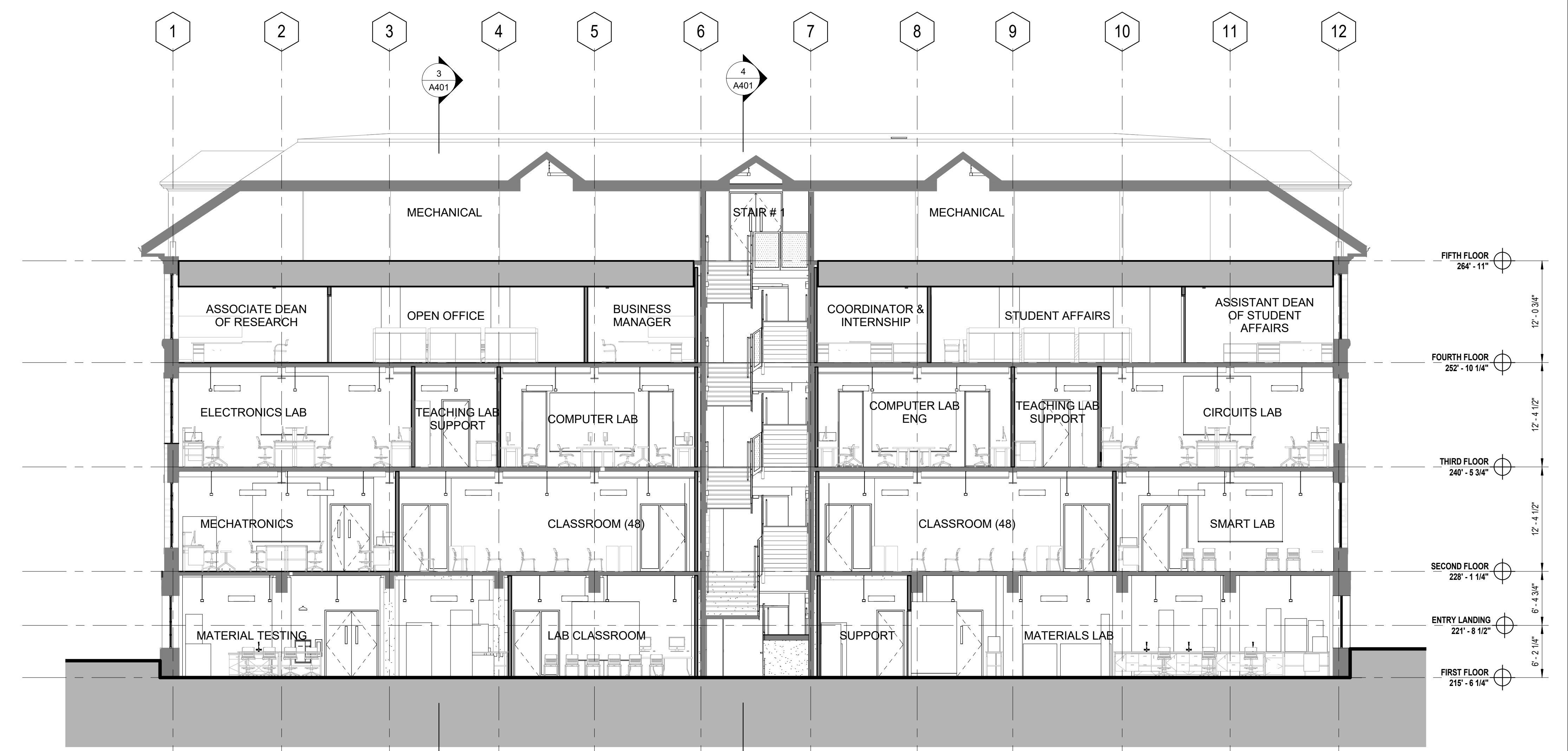
1/8" = 1'-0" 1 BUILDING SECTION SECTION @ EXISTING BUILDING LOOKING NORTH
