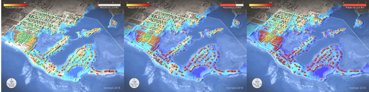
Visualizations of percent damage in the community of Matunuck RI, based on the Coastal and Environmental Risk Index (CERI).(1)
