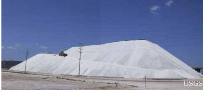
Figure 1 (left): Uncovered salt piles such as this will lose 20% of their salt to local waters each year.
