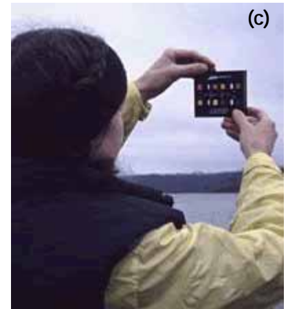
Fig. 2. (a) Laboratory quality pH meter and electrode with multiple reagents. (b) pH "pocket pal" for field monitoring of pH. (c) Volunteer uses a color comparator to assess pH (photo from EPA).
