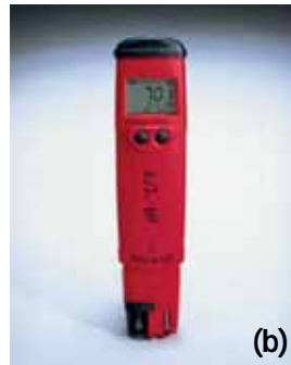
Fig. 2. (a) Laboratory quality pH meter and electrode with multiple reagents. (b) pH "pocket pal" for field monitoring of pH. (c) Volunteer uses a color comparator to assess pH (photo from EPA).
