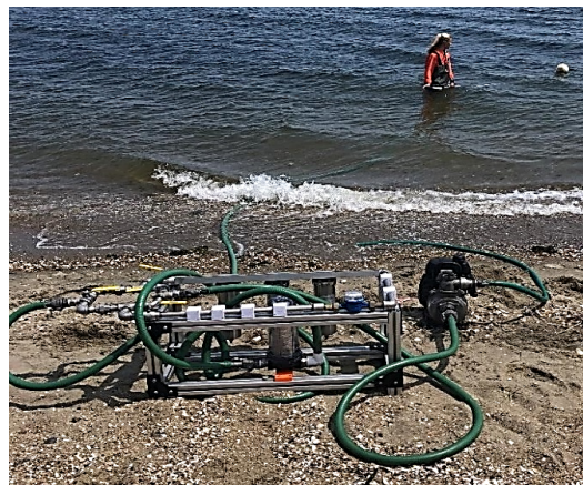
Ph.D. student Sarah Davis, who studies Biological and Environmental Sciences with a focus on microplastics in the environment. In this photo you can also see the pump-filter system in-use, testing microplastic particle recovery methods.
