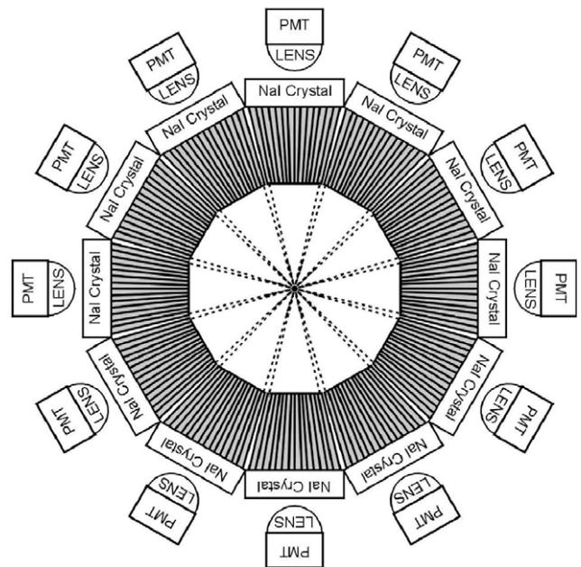
Fig. 6. Diagram of detectors and collimators.
