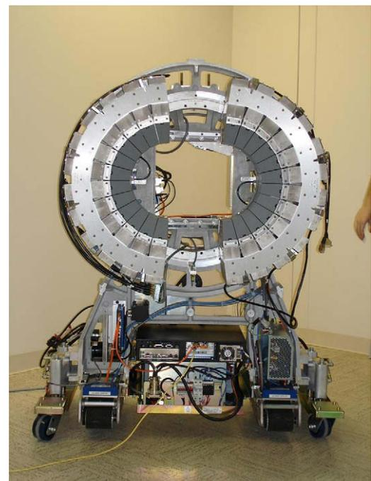
Fig. 10. Small, portable, high-resolution SPECT device (NeuroLogica Corp., Danvers, MA, USA) that can be brought into an epilepsy monitoring unit to scan a patient in the hospital bed.
