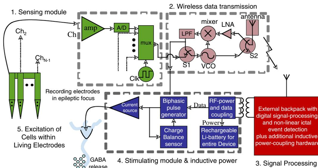
Fig. 18. A closed-loop living electrode prosthetic for epilepsy.
