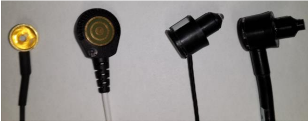
Figure 2. Disc EEG, tEEG electrodes and NIRS source and detector (from left to right)
