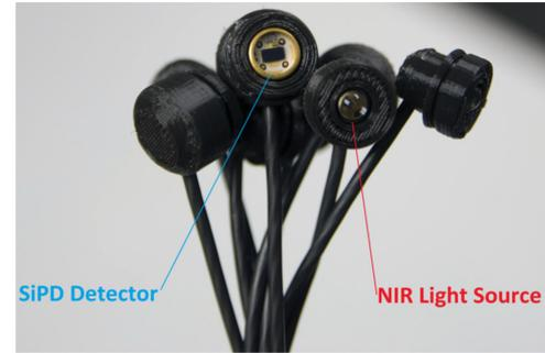
Fig. 5. 3D printed optode design. Optodes made of multi-wavelength LEDs (MTMD7885NN24) and Si-PD detectors (ODA-6 WB-500 M detectors).
