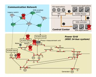
Figure 1: A simplified architecture of an SDN-enabled grid.
