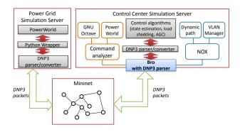
Figure 3: A cyber-physical co-simulation testbed.
