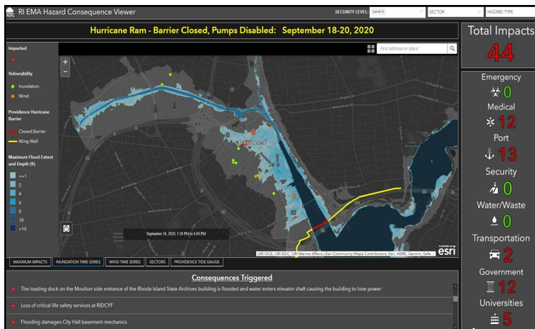
Fig. 4: Dashboard for the URI DHS Consequence Threshold project, coupling projected inundation with the number of assets impacted and specific consequences at each location.
