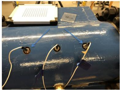
If there is black tape on the sensor wire then the wire cannot be disconnected from the sensor for easy removal. The torque wrench attachment should have a space for the wire to turn as the sensor is taken out. However if there is no black tape carefully turn and disconnect the sensor wire from the sensor then use the torque wrench to take the senor out.
