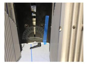
(k) Move the one camera at a time until the window is centered on the FastCam Viewer software as shown below. Usually with 85 mm lenses with a distance of
