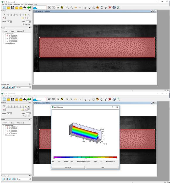
(t) Now click Data, click Coordinate Tools, and then Compute Cylindrical Transformation in the drop down menu. A window should pop up, hit Accept on the bottom right.
