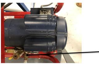
Pump Valve used to pressurize the tank
