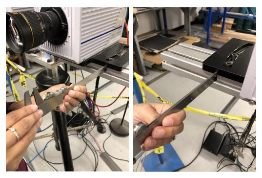
First extend the calipers out slightly. Next press the edge of the calipers into one side of the tripod mount and check the distance reading on the caliper. Repeat these steps again on the other side. If a very close reading is seen on both sides then the cameras are roughly parallel to the tripod mount. Finally lock the cameras in place.
