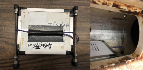
Next insert the extendable rods into the tube in tube and extend until they stay in place. Now take a plastic cord and tape one side on the back on the calibration grid. Run the other end through one of the sensor opening on the tube in tube and then back in through the second sensor opening. Tape the second end of the cord to the back of the calibration grid as shown below.
