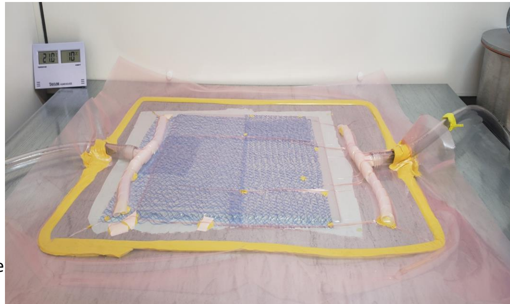
Fig. Experimental VARTM Setup
