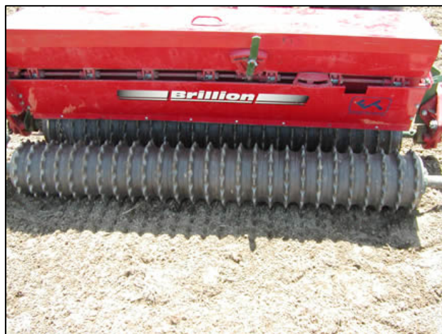
Brillion seeder with cultipacker. Photo courtesy of Cornell University Forage Breeding Project, Dr. Don Viands.
