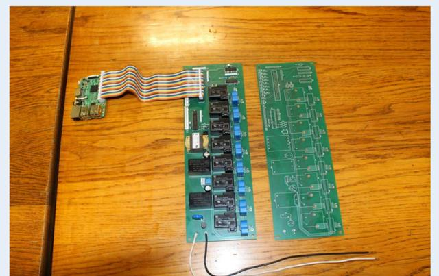
**Fig 1:** Assembled circuit board with microcontroller pictured next to the empty printed circuit board.
