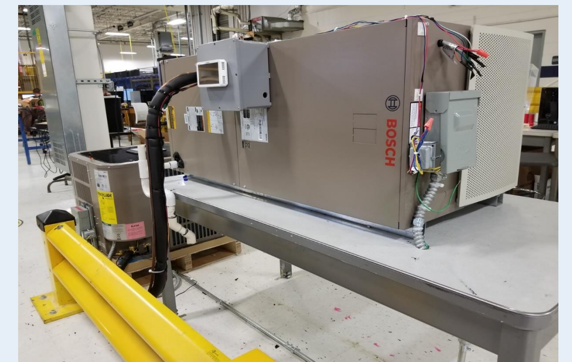
Figure 1 – IDS unit – Air Handler (right) & Condenser (left)
