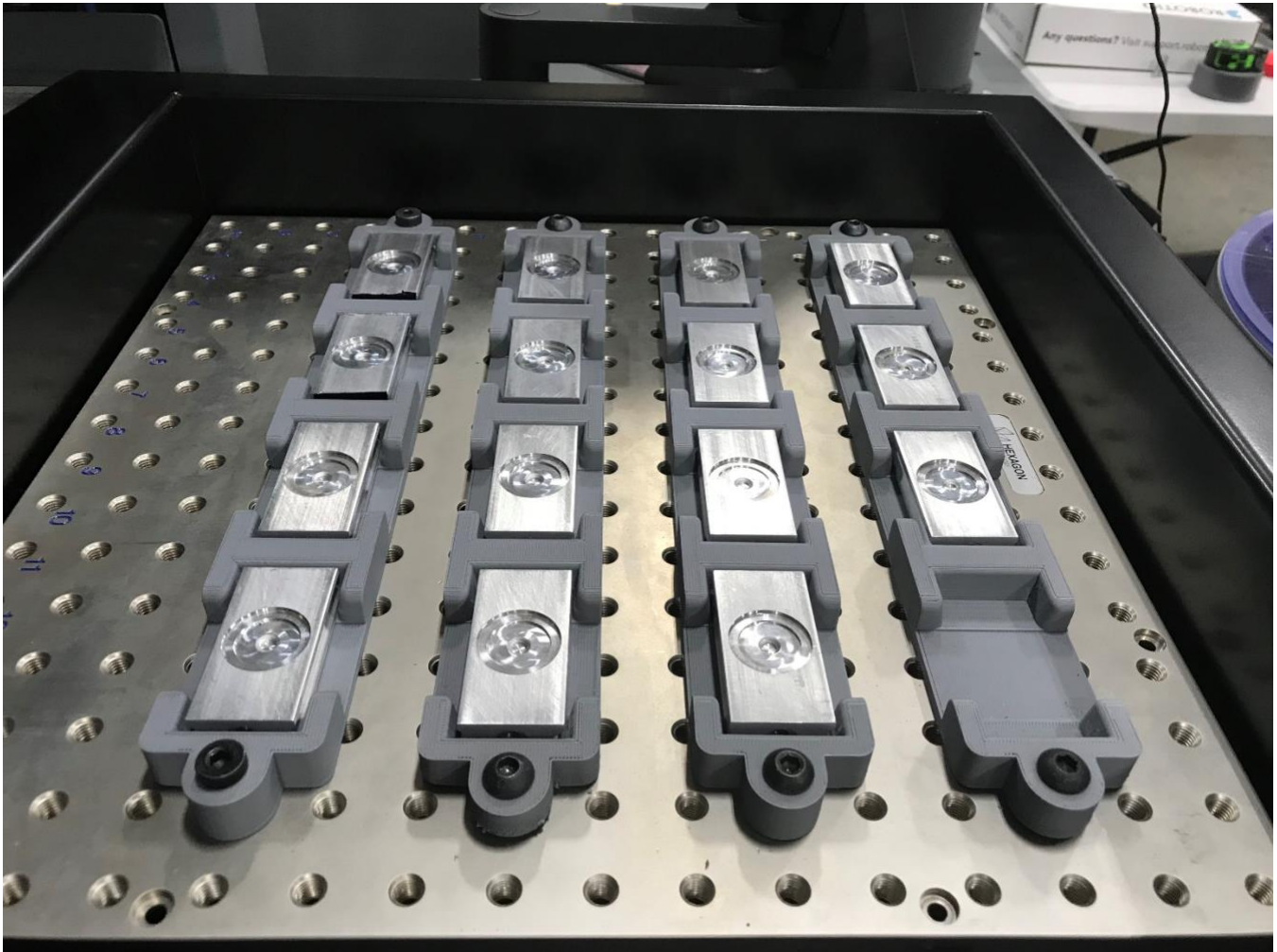
View of the air bearing pallet arrangement
