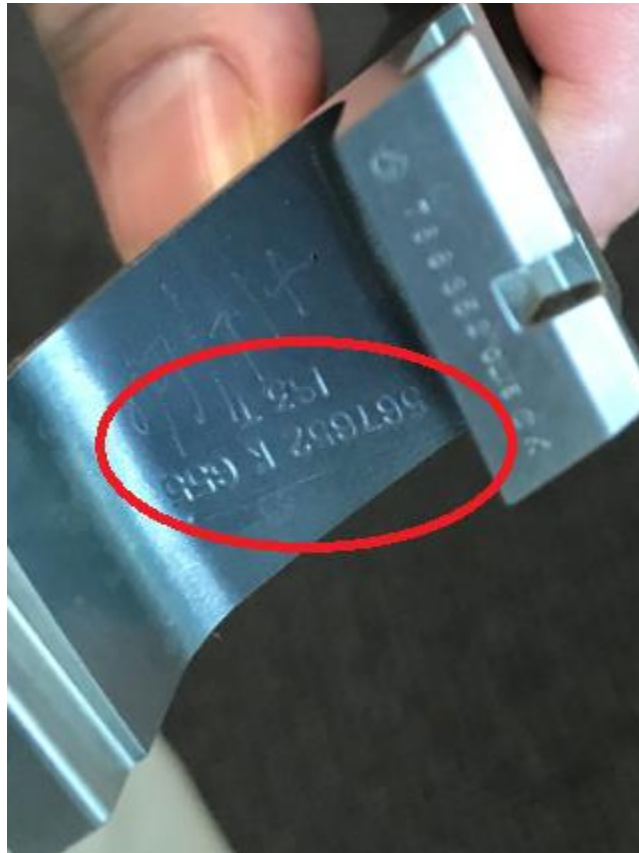
Example of a difficult serial number to capture without human assistance. (Serial number is on the base of a jet engine vane)
