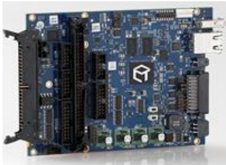
Figure 1: Scan Master Controller. Galvo Scanner and Laser controller.
