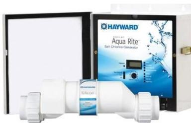
Hayward manufactures several hundred thousand of [AquaRite](#) chlorine generator systems and "salt cells". These apply DC current to Ruthenium coated Titanium plates to generate chlorine gas in an electrolysis reaction.
