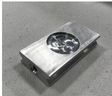
Air bearing (internal CMM part)
