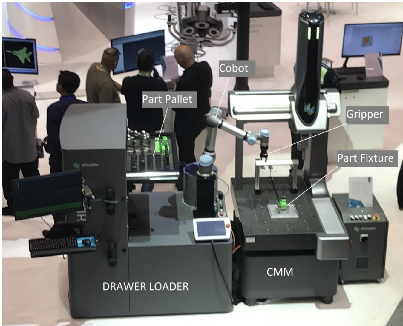
Automated Inspection System Overview
