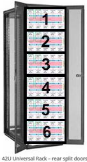
Figure 1: Front View of test system rack. 6 main boards will be mounted to the front for easy DUT (device under test) accesibility. Test equipment such as dc-dc supplies and data acquisition equipment will be mounted in the rear.
