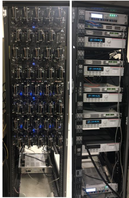
Figure 1: Front and Back view of test system rack. 4 of 6 main boards are mounted to the front for easy DUT accessibility. DC-DC supplies and data acquisition equipment are mounted in the rear.
