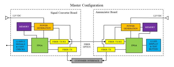
Proper design and application of fiber optic annunciator system will lead to a highly secure system. Engineers will choose proper components, design, programming and install an appropriate fiber optic cable system, test components selected and the ultimate design to be immune to any interference.
