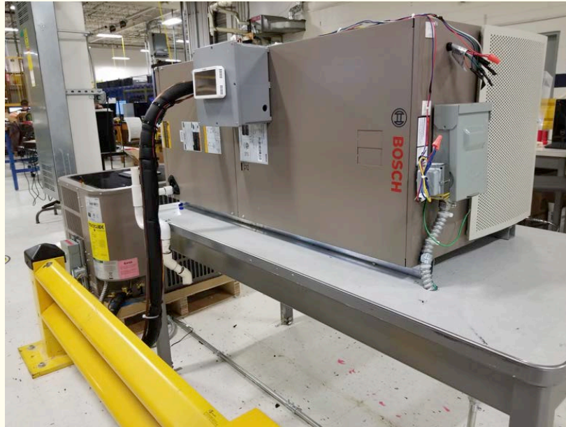
Fig 1: IDS unit – Air Handler (right) & Condenser (left)
