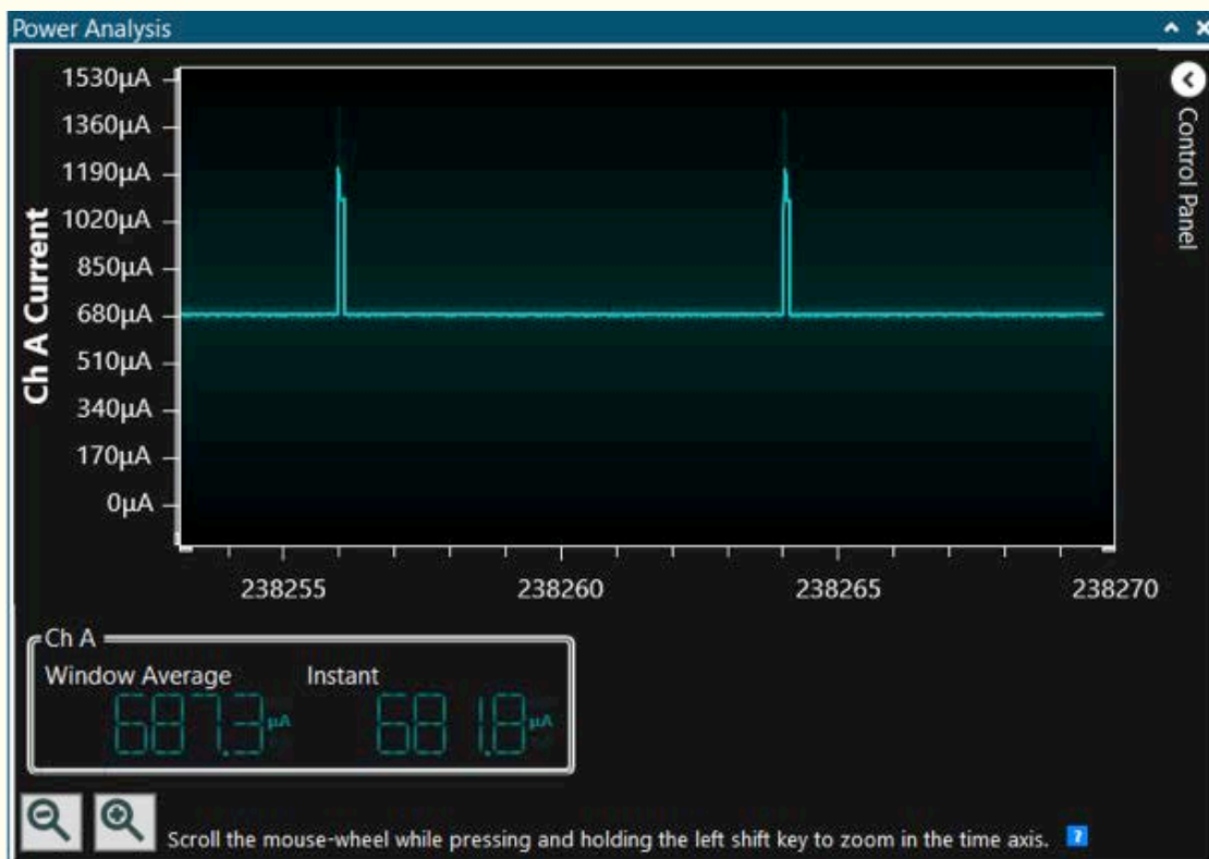
Fig 3: Power Consumption Graphs of Poolside Sensor Unit in Awake Mode vs. Sleep Mode
