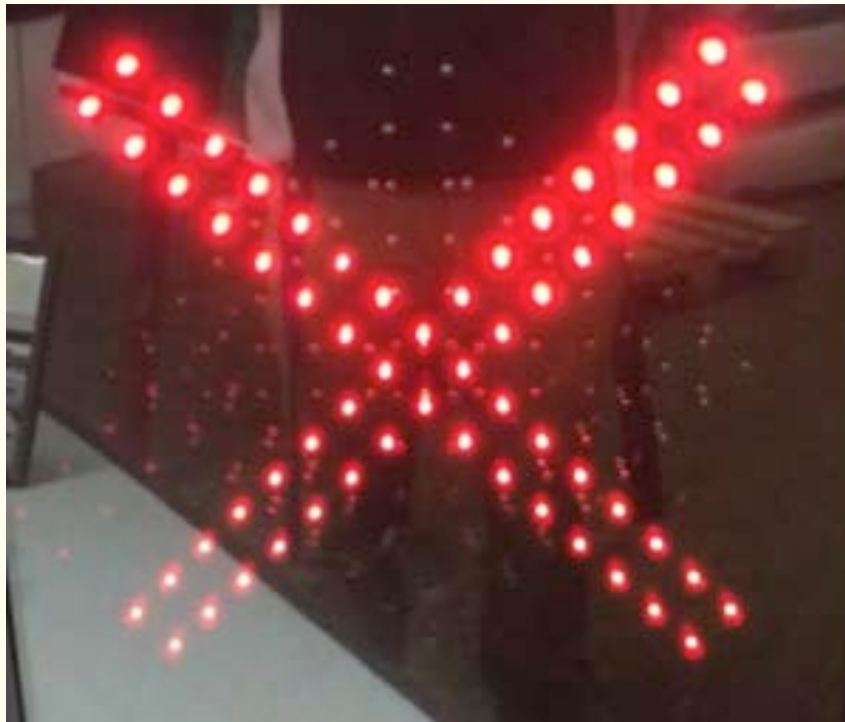
Fig 1: Blank Out-Signs that are to be retrofitted with the cellular module to allow connection to the server for receiving a new message.
