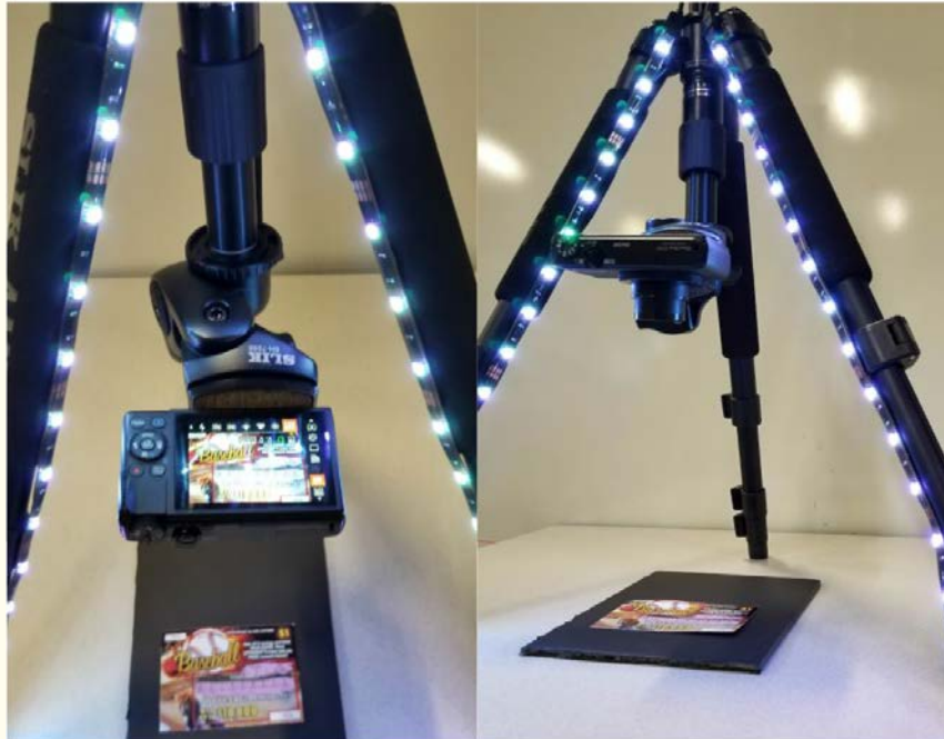
Fig 1: Inverted Tripod Camera Display used to collect RAW images.
