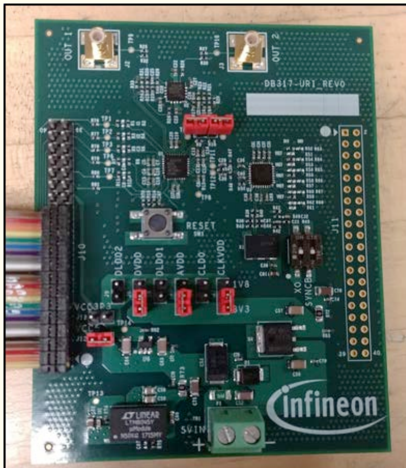
Fig 2: Waveform Generator Board
