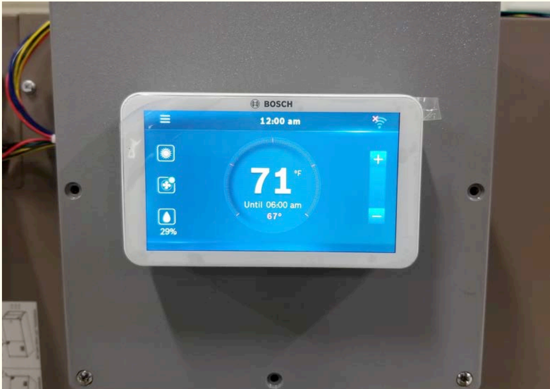
Fig 3: Housing with touchscreen IDS control
