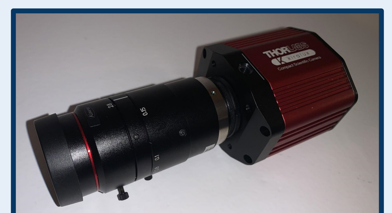
Fig.4: CS505MU Camera with MVL50TM23 Lens
